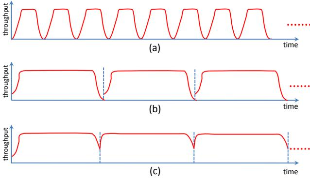
**Figure 6:** Different strategies for parallel collision query using work queues. (a) Naive way: repeat the single collision query algorithm one by one; (b) Work queues are initialized by some BVTT root nodes and we repeat the process until all queries are performed. (c) is similar to (b) except that new BVTT root nodes are added to the work queues by the pump kernel, when there is not sufficient number of tasks in the queue.
