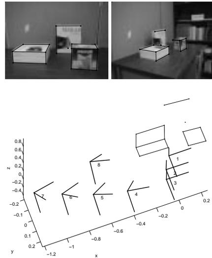
**Figure 1:** Two sample views of the scene and recovered 3D structure of the scene and camera motion.
