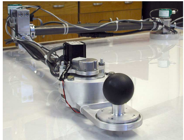
Figure 2: A 2-dof cobot, which presents stiff yet smooth constraint paths to a human user grasping the handle. The wide, low design allows large constraint forces and a full range of human arm motion.
