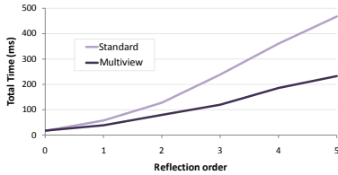
Fig. 8: Multiview performance: Multi-view ray tracing out performs standard ray tracing for scenes (80k triangle scene shown) with many specular views. The multi-view timings include the time cost of all necessary sorting and reordering.
