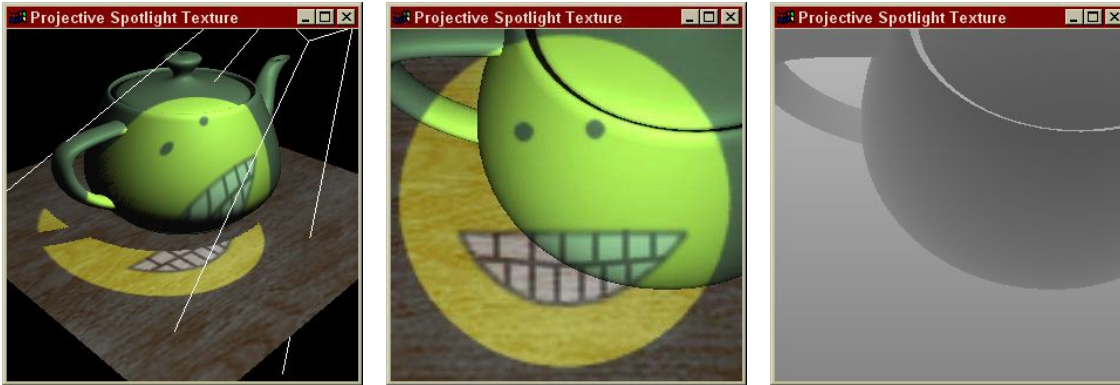
Figure 2. A shadow mapped scene rendered from the eye's point of view (left), the scene as rendered from the light's point of view (center), and the corresponding depth/shadow map (right).
