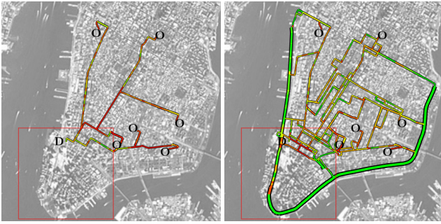
Figure 6: An example of the MSSD scenario: in which vehicles are spawned at various origin points and drive to a single destination. On the left is the mean velocity field of the fastest-path baseline router, and on the right is the mean velocity field resulting from our method. The destination point was chosen randomly inside the destination region, designated by the red rectangle. The origin points were chosen randomly outside this region with the additional constraint that they be at least 1km away from the destination. The mean velocity is shown as a color ranging from red, 0 m/s, to green, 13 m/s, the speed limit for most of the roads.
