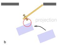
projection functions move the bounding box in order to put door handles into reaching area of robot hands.
