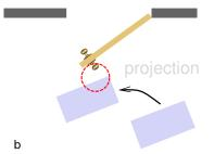
projection functions move the bounding box in order to put door handles into reaching area of robot hands.
