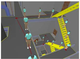
**Plate 3:** A composite image of an avatar following an automatically generated, collision free path through the power plant model.
