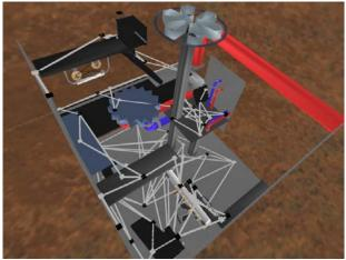
**Plate 1:** An automatically computed navigation roadmap for a small factory environment consisting of 10 thousand triangles.
