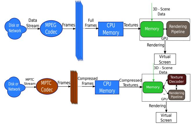
**Figure 6:** Top figure shows the traditional video rendering pipeline for VR. Bottom figure shows the MPTC decompression and video rendering method using compressed textures for VR. Our pipeline provides various benefits over the current pipeline.
