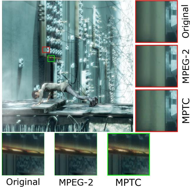
**Figure 8:** Zoomed in visual comparison for a frame from the elephant benchmark video. An interesting part ( $32 \times 32$ ) of a frame is cropped and zoomed to compare different formats and is compared with the original.
