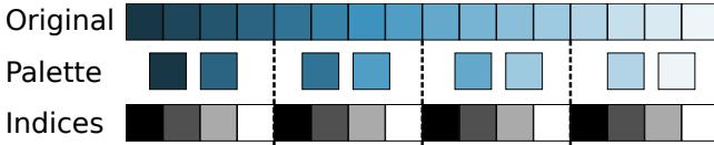
**Figure 3:** Our method (MPTC) uses the block level coherency of the image features to find redundancies in index data. In this example, a gradient duplicates the same indices four times across the compressed data. Many images exhibit block-level coherence for image features that are larger than a block. This assumption comes from the per-block palette endpoints interpreted as a low-frequency approximation of the original image while the indices represent the high-frequency modulation values.
