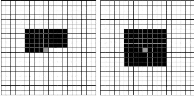
**Figure 5:** The search windows used during recomputation of the index data in our approach (MPTC). (left) The gray block is the current block being re-encoded; the blocks marked in black are the search blocks for a possible index data match for the gray block in an intra-block search. (right) The blocks marked in the black are the search blocks for predictive-block search in the previous frame. The gray block shows the position of the block being re-encoded in the current frame.
