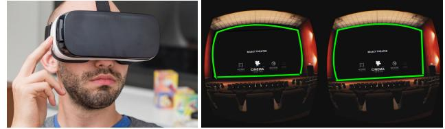
**Figure 1:** (left) Person watching a movie in Galaxy Gear VR. (right) The different view points are rendered for each eye on the user's mobile screen. We use our novel MPTC algorithm to compactly represent the video frames and decode them using commodity GPUs. MPTC reduces CPU-GPU bandwidth requirements and can result in  $3\text{--}4\times$  improvement in the frame rate over prior representations on HMDs using a desktop.
