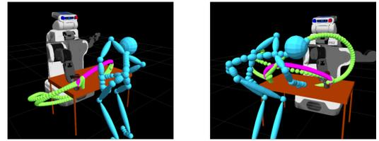
Fig. 9: Parallel replanning in dynamic environments with a human obstacle. The planner optimizes multiple paths which are smooth and avoid collision with the obstacle. Each colored path corresponds to a different search in the configuration space. The optimal path for each case is shown in purple.
