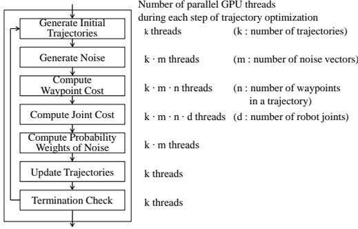
Fig. 4: The detailed breakdown of GPU trajectory optimization. It starts with the generation of  $k$  initial trajectories. From these initial trajectories, the algorithm iterates over stochastic optimization steps. The waypoint costs include collision cost, end effector orientation cost, etc. We also compute joint cost, which might include smoothness costs or the cost of computing the torque constraints. The current trajectory cost is repeatedly improved until the time budget runs out.
