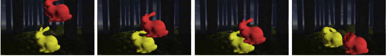
Figure C.1: Proximity Computations on Deforming Models: We use our interactive distance field computation for separation and penetration distance for dynamic simulation of deforming bunnies. Each bunny consists of 2K triangles and we compute localized distance fields on a 256^3 grid for the simulation shown in this sequence. The average distance field and proximity query takes 120ms on a 3.2 GHz Pentium IV PC with NVIDIA GeForce 7800 GPU.
