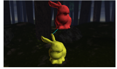
Figure 3: Separation Distance Computation between deforming bunnies: Average query time=120ms, grid resolution= 256^3 .
