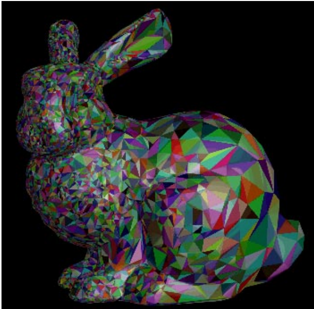
Figure 9: An adaptive simplification for the bunny model. \epsilon varies from 1/64% at the nose to 1% at the tail.
