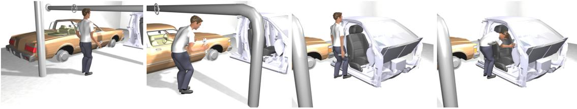
Figure 5: Walking & Bending: The human model walks towards the car, avoiding some obstacles. It bends and stretches to put the tool inside the car. The latter is a highly constrained environment and we need to perform whole-body planning to generate such motions.
