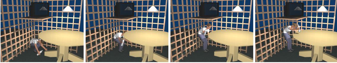
Figure 3: Object Retrieval: In this benchmark, the human model stands up and places the object on the table. The overall motion involves use of many DOFs and the resulting path is collision-free.
