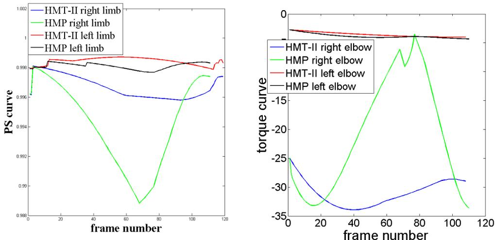
Figure 7: Comparison of posture similarity (PS, left) and torque variation (TV, right) between HMP and HMT-II, in the Object Retrieval benchmark.
