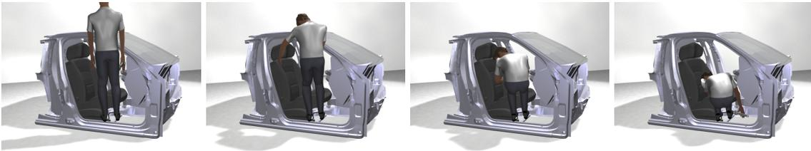
Figure 6: More bending: The human bends and stretches to put the tools under the chair. This environment is far more constrained than the one of Walking & Bending (Fig. 6). The whole-body planning becomes even more challenging in such constrained environments.
