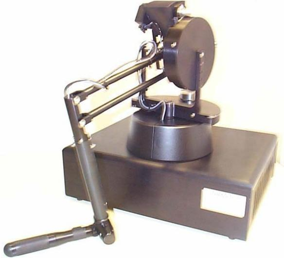
Fig. 17. 6-DOF Haptic Device: The PHANTOM of SensAble Technologies
