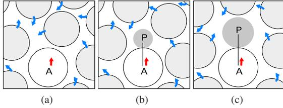
**Figure 2: Aggression:** Agent  $A$ 's desired direction is blocked. As  $A$ 's urgency increases, its aggression proxy,  $P$ , grows and the other agents move to avoid it, leaving a space for  $A$  to move into.
