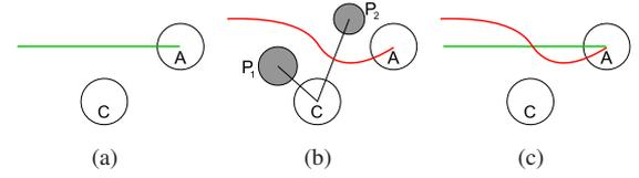
**Figure 1:** Responses of an agent  $A$  encountering a composite agent  $C$ . (a) The green line shows the original planned path taken by  $A$ . (b) In the presence of the proxy agent of  $C$ ,  $A$  takes the red path and avoids collision with  $P_1$  and  $P_2$ . (c) Comparison of the paths.
