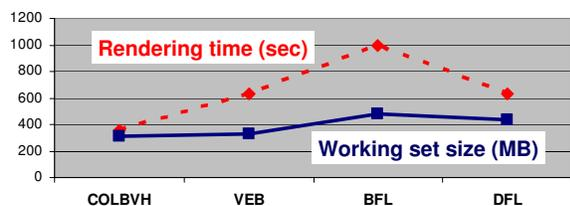
**Figure 8: Performance of Ray Tracing:** Average render time and the size of working set during ray tracing of the Lucy model with 28 million triangles are shown with different layouts. By using the cache-oblivious layout, we are able to achieve 77%–180% improvement in the performance of ray tracing and reduce the working set size by 7%–55%.
