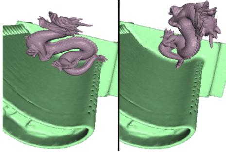
**Figure 5: Dynamic Simulation between Dragon and Turbine Models:** This image sequence shows discrete positions from our dynamic simulation between dragon and CAD turbine models. We are able to achieve 38%–215% performance improvement in collision detection by using our cache-efficient layouts of the OBB-tree over other tested layouts.
