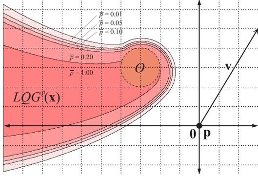
Fig. 4. The LQG-Obstacle  $\mathcal{LQG}^{\bar{p}}(\hat{\mathbf{x}})$  in the same configuration as in Fig. 2 accounting for motion and sensing uncertainty of the robot (see Section V-B). The conservative approximation of Eq. (25) is shown for various values of the probability bound  $\bar{p}$ . For  $\bar{p} = 1$ , it is equivalent to the LQR-Obstacle.
