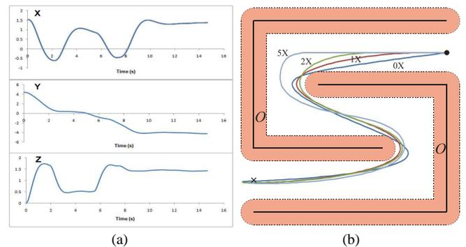
Fig. 8. (a) The  $x$ ,  $y$ , and  $z$  position over time of the quadrotor in the *3-Window* scenario (see Fig. 1). (b) The  $xy$ -projections of the maximum likelihood traces of the quadrotor in the *S-Maze* scenario (see Fig. 7) for 0, 1, 2, and  $5\times$  the realistic amount of uncertainty.
