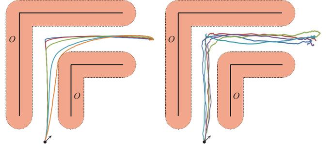
Fig. 5. Controlling the robot (see Section V-B) using LQG-Obstacles in the same environment as Fig. 3. (a) Traces of maximum likelihood executions for  $\bar{p} = \{0.01, 0.02, 0.03, 0.05, 1\}$ . (b) Traces of five actual executions with synthetic motion and observation noise for  $\bar{p} = 0.01$ .
