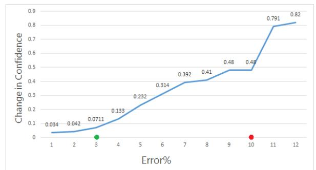
Fig. 7: Change in confidence vs percentage of error. This was performed to evaluate the variation in the confidence function with respect to the tracking error. This classification is used to determine whether the tracker accuracy for a pedestrian is low, indicating that we need to switch to a more accurate tracker.
