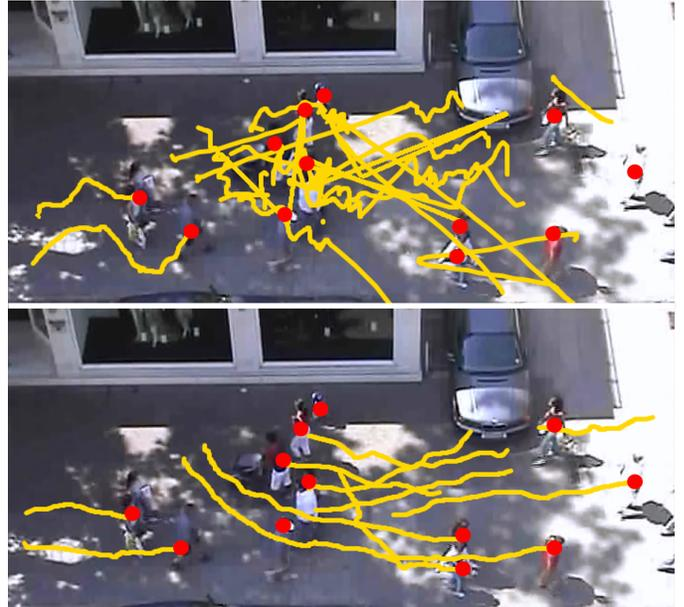
Fig. 1: Comparing AdaPT (bottom) with the Mean-shift tracker [15] (top). AdaPT's frame rate in this scene is 27 fps, as compared to 31 fps for mean-shift tracker. However, our algorithm is able to accurately compute all the trajectories, shown as yellow lines. Red circles represent ground truth. (Dataset - zara01 [20])
