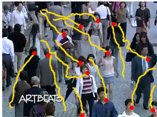
Fig. 9: AdaPT’s frame rate in this scene is 27 fps, tracking 14 pedestrians accurately in real-time. (Dataset CRW116: Web Stock Footage from Collection “Pedestrians from above”)
