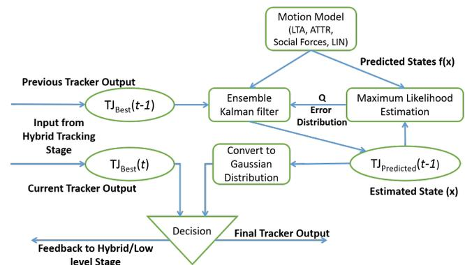
Fig. 5: Overview of the High-Level Motion Model Augmentation Stage. This stage draws input from the Confidence Estimation stage, learns model parameters and improves tracking by providing feedback. The feedback is bidirectional and the model is re-trained after a fixed number of frames. The ‘Decision’ module is a parameter that can be modified depending on how much importance the motion model is given.
